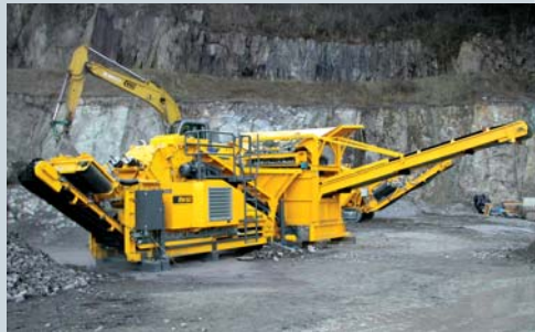
Highest possible throughput in crusher with low wear thanks to pre-screening fine material
