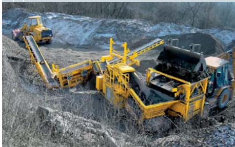
Highest efficiency - as stand-alone screen or with RM crusher as complete on-site recycling centre
