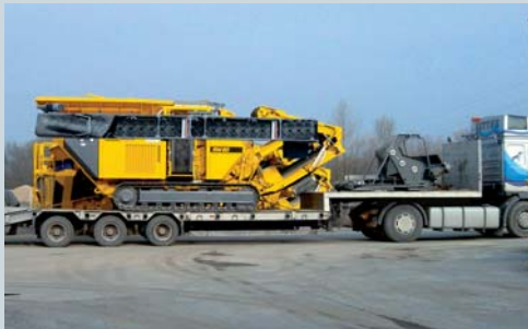
Profit from mobility: crusher and OS80 (including return belt) delivered with just one transporter
