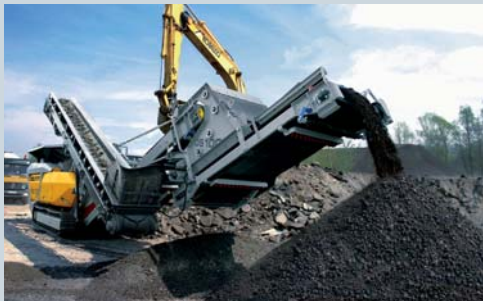
Unrestricted mobility on-site for RM crusher mounted on crawler gear plus oversized grain system
