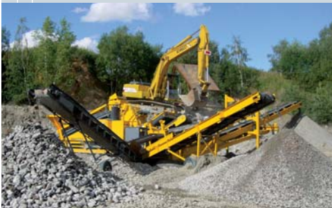
Throughput capacity up to 100 t/h with double-deck version – highest separation accuracy
