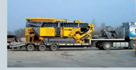
Both the crusher and OS80 / OS100 can be transported with just one low-loader and are ready for operation within 20 minutes of arrival on site.
