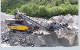
The refeeding belt provides a closed circuit system maintaining unrestricted movement of the crusher
